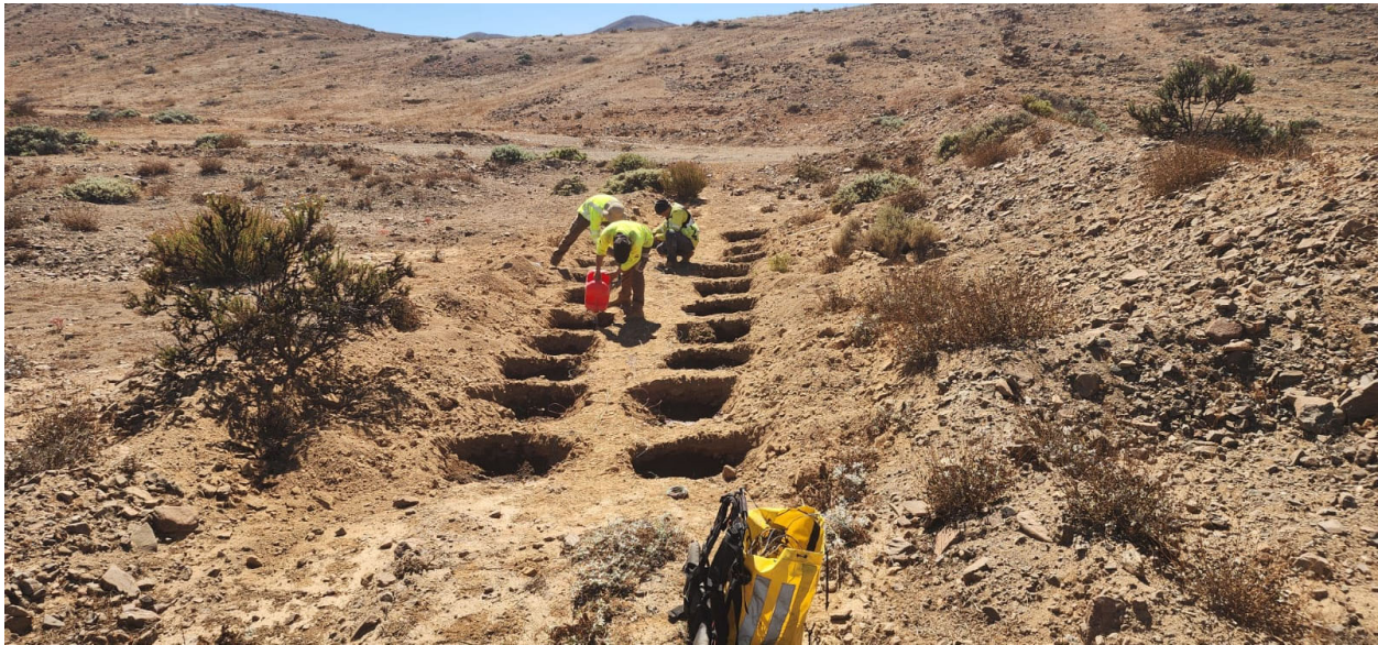
Figure 3 - IP crew laying out chargeability cables at the northern grid location.
