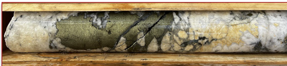
Chalcopyrite in brecciated quartz vein; FAR-22-019, 86m
