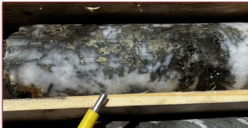
Chalcopyrite primary; FAR-22-020: photo within 139.9-147.7m 7.8m @ 0.83% Cu/0.09% Co/0.19g/t Au
