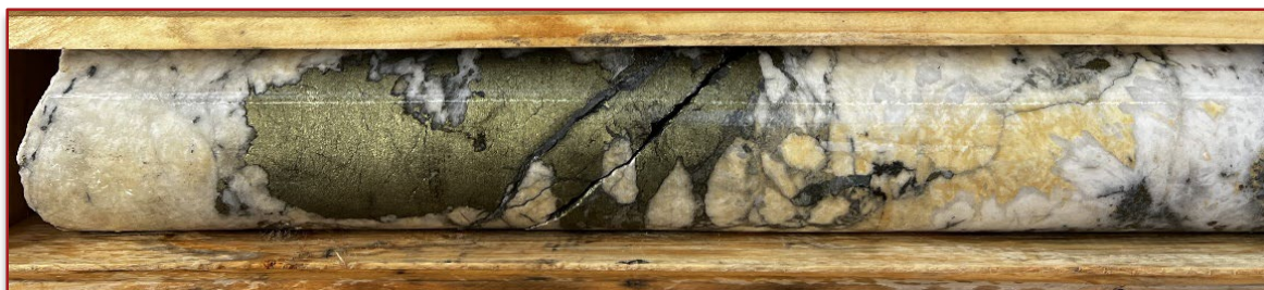
Chalcopyrite in brecciated quartz vein; FAR-22-019 photo within 86-88.8m 2.8m @ 0.9% Cu/0.02% Co/0.04g/t Au
